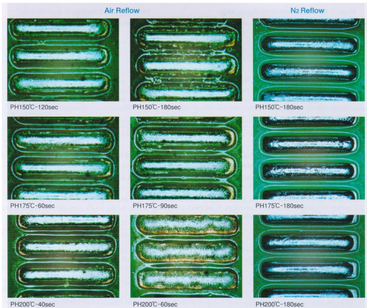
Photo 3 Effect of Different Pre-Heat Conditions (SnAgCu-RMA)
